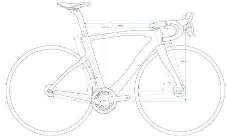
CE: SEATTUBE CENTER - END, CC: SEATTUBE CENTER - CENTER, L: TOP TUBE CENTER - CENTER, A [°]: SEAT TUBE ANGLE, B [°]: HEADTUBE ANGLE, P: CHAINSTAY T: HEADTUBE, D: BB DROP, R: FORK RAKE, G: FORK HEIGHT, REACH, STACK
